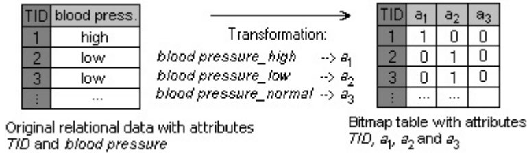
Fig. 2. Transformation of relational data into an efficient bitmap representation for attributes with no-binary domains.
